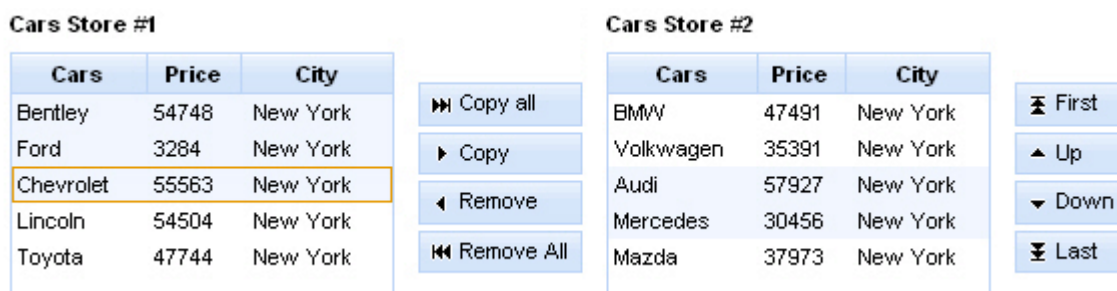
Figure 6.171. <rich:ListShuttle> component
