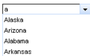
Figure 6.130. <rich:comboBox> with "selectFirstOnUpdate" attribute.
